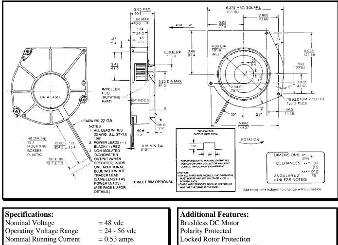
Nominal Running Current= 0.53 ampsLocked Rotor Current= 1.0 ampsRunning Power= 25.4 wattsAverage Speed= 2500 rpmBearings= BallAir Flow= 59 CFMAcoustic= 57.0 dBA
